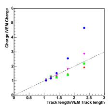
**Figure 2.** The points show for 5 different angles  $(20^{\circ}, 35^{\circ}, 45^{\circ}, 56^{\circ})$  and  $(30^{\circ})$  the charge measured in the 3 PMTs (triangle up, square, circle) as well as the total charge on the sum of the PMTs (triangle down), with respect to the track length in the tank. All quantities are normalize to the VEM corresponding values for comparison.
