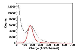
**Figure 1.** The muon charge histogram triggered by the scintillators for the  $Q_{VEM}$  and by the coincidence of the 3 PMTs for the  $Q_{VEM}^{peak}$ . In the left for the sum of the 3 PMTs, and in the right for a single PMT.
