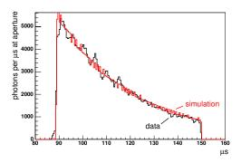
**Figure 4.** Light profile at the aperture of the Los Leones FD of a vertical CLF laser shot recorded under extremely clear atmospheric conditions. This simplified simulation assumes an aerosol-free atmosphere. The horizontal axis corresponds to the time since the laser fired.
