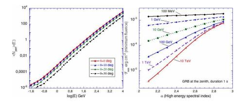
Figure 1. Left: Mean number of detected particles in a tank as a function of the photon primary energy for different zenith angles. Right: Minimum fluence between 10 MeV and  $E_{max}$  for a GRB to be observable as a function of the spectral index.
